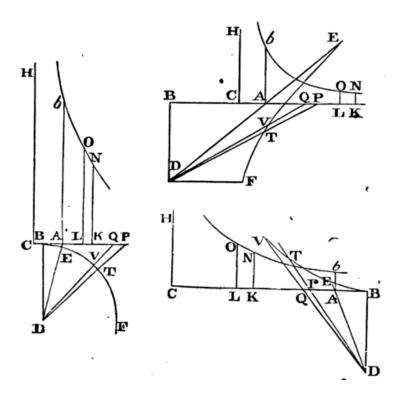
body is descending, otherwise on the contrary. Erect Ab, which make to DB as DB<sup>2</sup> to 4BAC: and to the rectangular asymptotes CK, CH, describe the hyperbola bN; and, erecting KN perpendicular to CK, the area AbNK will be augmented or diminished in an arithmetical progression, while the forces CK are taken in a geometrical progression. I say, therefore, that the distance of the body from its greatest altitude is as the excess of the area AbNK above the area DET.
