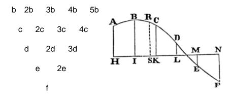
Case 1. If HI, IK, KL, &c., the intervals of the points H, I, K, L, M, N, &c., are equal, take *b*, *2b*, *3b*, *4b*, *5b*, &c., the first differences of the perpendiculars AH, BI, CK, &c.; their second differences *c*, *2c*, *3c*, *4c*, &*c*.; their third, *d*, *2d*, *3d*, &c., that is to say, so as AH - BI may be = *b*, BI - CK = 2*b*, CK - DL = 3*b*, DL + EM = 4*b*, - EM + FN = 5*b*,
