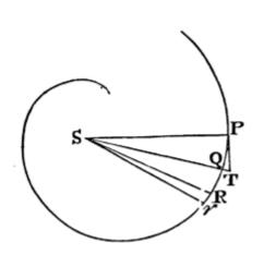
Let that spiral be PQR. From the velocity, with which the body goes over the very small arc PQ, the time will be given; and from the altitude TQ, which is as the centripetal force, and the square of the time, that force will be given. Then from the difference RS*r* of the areas PSQ and QSR described in equal particles of time, the retardation of the body will be given; and from the retardation will be found the resisting force and density of the medium.
