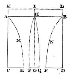
Cor. 7. If in the middle of the hole EF there be placed the little circle PQ described about the centre G, and parallel to the horizon, the weight of water which that little circle sustains is greater than the weight of a third part of a cylinder of water whose
