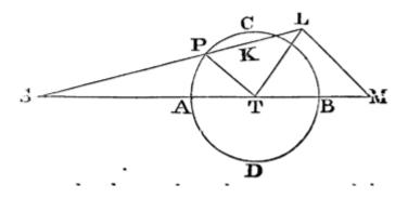
Let S represent the sun, T the earth (419, 420), P the moon, PAGB the moon's orbit. In SP take SK equal to ST and SL to SK in the duplicate ratio of SK to SP. Parallel to PT draw LM; and, supposing the mean quantity of the circum-solar force directed towards the earth to be represented by the distance ST or SK, SL will represent the quantity thereof directed towards the moon. But that force is compounded of the parts SM, LM; of which the force LM and that part of SM which is represented by TM,
