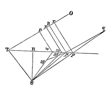
*rp* meeting TP in *p*. Then through the point S*p* draw the line S*q* equal to  $\frac{M^2 \times N}{Or^2}$ . In like manner draw three or more right lines S2*q*, S3*q*, &c., and a regular line *q*2*q*3*q*, drawn through all the points *q*2*q*3*q*, &c., will cut the right line TP in the point P, from which the perpendicular PR is to be let fall. Q.E.F.
