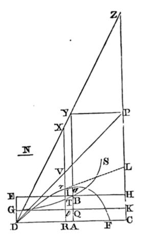
Let the projectile go from any place D in the direction of any right line DP, and let its velocity at the beginning of the motion be expounded by the length DP. From the point P let fall the perpendicular PC on the horizontal line DC, and cut DC in A, so that DA may be to AC as the resistance of the medium arising from the motion upwards at the beginning to the force of gravity; or (which comes to the same) so that the rectangle under DA and DP may be to that under AC and CP as the whole
