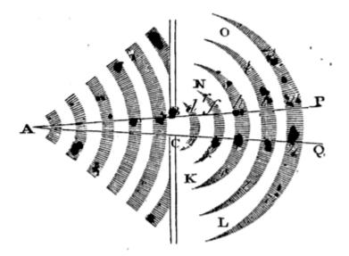
Case 1. Let a motion be propagated from the point A through the hole BC, and, if it be possible, let it proceed in the conic space BCQP according to right lines diverging from the point A. And let us first suppose this motion to be that of waves in the surface of standing water; and let *de, fg, hi, kl,* &c., be the tops of the several waves,
