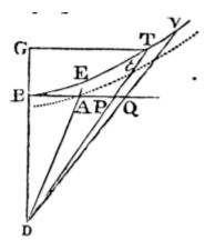
Case 3. Let AP be the velocity in the descent of the body, and  $AP^2 + 2BAP$  the force of resistance, and  $BD^2 - AB^2$  the force of gravity, the angle DBA being a right one. And if with the centre D, and the principal vertex B, there be described a rectangular hyperbola BETV cutting DA, DP, and DQ produced in E, T, and V; the sector DET of this hyperbola will be as the whole time of descent.
