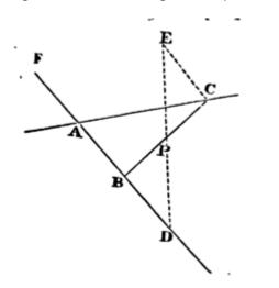
From the given point P suppose any right line PD to be drawn to either of the right lines given, as AB; and produce the same towards AC, the other given right line, as far as E, so as PE may be to PD in the given proportion. Let EC be parallel to AD. Draw CPB, and PC will be to PB as PE to PD. Q.E.F.
