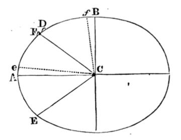
A is in the middle between the points E, F, and the point D in the middle between the points *e*, *f*, if the difference of the heights CA, CB, represent the quantity of the tide in a very deep sea surrounding the whole earth, the excess of the height CA above the height CE or CF will represent the quantity of the tide in the middle of the sea EF,
