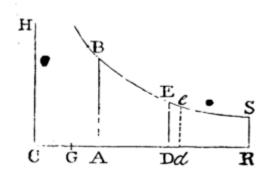
In the asymptote CD let there be given the point R, and, erecting the perpendicular RS meeting the hyperbola in S, let the space described be expounded by the hyperbolic area RSED; and the velocity will be as the length GD, which, together with the given line CG, composes a length CD decreasing in a geometrical progression, while the space RSED increases in an arithmetical progression.
