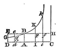
The body ascending, let the gravity be expounded by any given rectangle BACH; and the resistance of the medium, at the beginning of the ascent, by the rectangle BADE, taken on the contrary side of the right line AB. Through the point B, with the rectangular asymptotes AC, CH, describe an hyperbola, cutting the perpendiculars DE, *de*, in G, *g*; and the body ascending will in the time DG*gd* describe the space EG*ge*; in the time DGBA, the space of the whole ascent EGB; in the time ABKI, the
