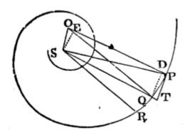
For from the right angles OPQ, OQR, subduct the equal angles SPQ, SQR, and there will remain the equal angles OPS, OQS. Therefore a circle which passes through the points OSP will pass also through the point Q. Let the points P and Q coincide, and this circle will touch the spiral in the place of coincidence PQ, and will therefore cut the right line OP perpendicularly. Therefore OP will become a diameter of this circle, and the angle OSP, being in a semi-circle, becomes a right one. Q.E.D.
