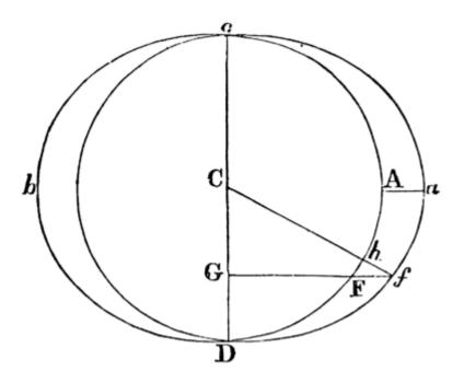
Let Aa (in the following figure) represent that excess of height of 9 inches at A, and hf the excess of height at any other place h; and upon DC let fall the perpendicular fG, meeting the globe of the earth in F; and because the distance of
