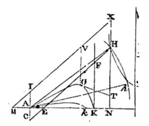
Therefore if a body projected from the place A, in the direction of the right line AH, describes the hyperbola AGK and AH produced meets the asymptote NX in H, and AI drawn parallel to it meets the other asymptote MX in I; the density of the medium in A will be reciprocally as AH, and the velocity of the body as  $\sqrt{\frac{AH^2}{AI}}$ , and the resistance there to the force of gravity as AH to  $\frac{2nn+2n}{n+2} \times AI$ . Hence the following rules are deduced.
