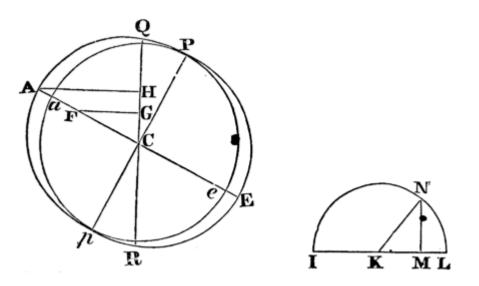
IL let fall the sines NM. Then the sums of the squares of all the sines NM will be equal to the sums of the squares of the sines KM, and both sums together will be equal to the sums of the squares of as many semi-diameters KN; and therefore the sum of the squares of all the sines NM will be but half so great as the sum of the squares of as many semi-diameters KN.
