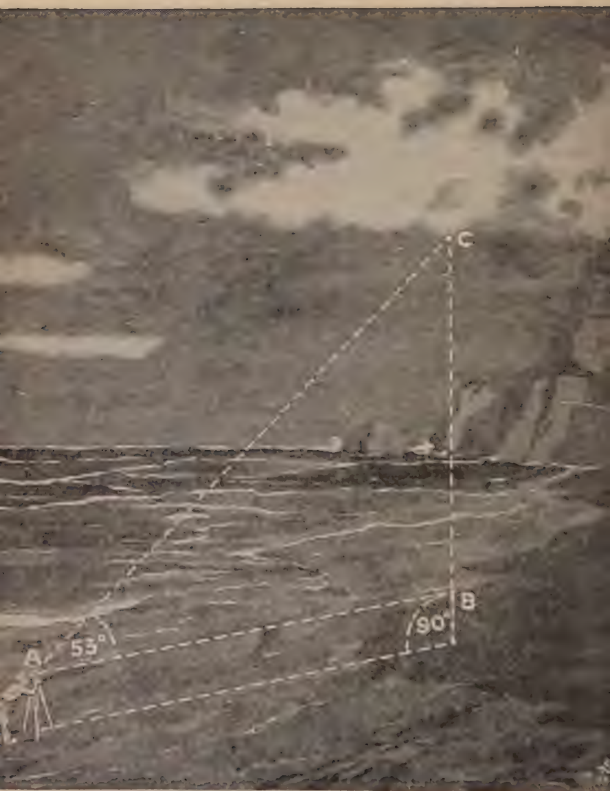
Finding the height of a cloud by trigonometry.
